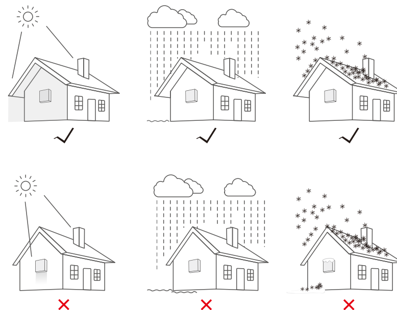
▲ Figure 4.1 Recommended Installation locations
